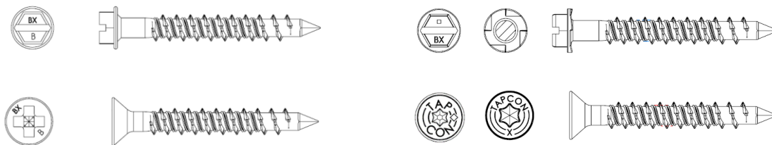
FIGURE 2—TAPCON ANCHORS WITH ADVANCED THREADFORM TECHNOLOGY ANCHORS
