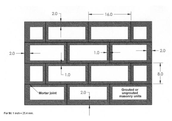
FIGURE 5—ANCHOR LOCATIONS (LIGHT COLOR AREAS) FOR INSTALLATION IN MASONRY UNITS (ALL DIMENSIONS IN INCHES)
